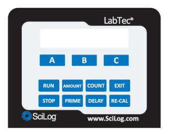
The front panel consists of a user interface, which includes an alphanumeric display and a membrane keypad to select operational modes and alarm settings. The display is a two line, 20 character each, liquid crystal display (LCD). The display is backlit to allow easy viewing over a wide range of lighting conditions.
