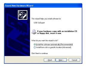
Insert the CD containing the LabTec Operating Manual into the PC, choose "Install the software automatically" and click "Next". The following screen appears:
