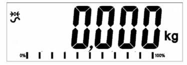
• The scale has an automatic re-zeroing function to account for minor drifting or accumulation of material on the platform. However you may need to press the [→0←/Esc] key to re-zero the scale if small amounts of weight are shown when the platform is empty.
