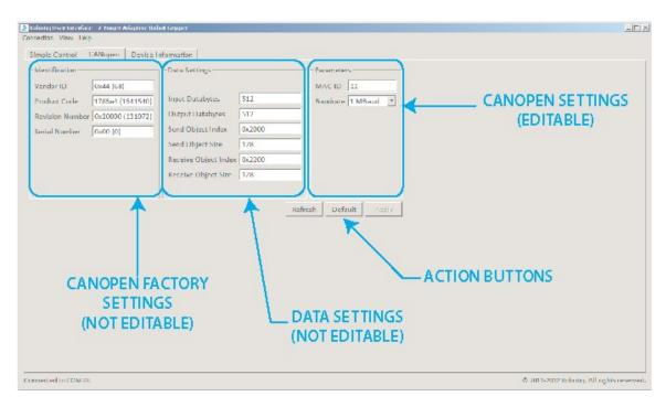
Fig. 6-7: Default screen of the Configuration Tool with CANopen
