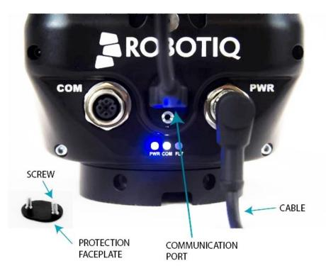
Fig. 3-5: Completed USB connection of the 3-Finger Adaptive Robot Gripper.
