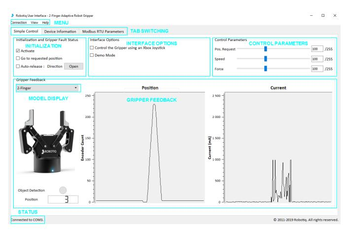
Fig. 5-9: The Simple Control tab for the Robotiq User Interface for 2-FingerGripper and Hand-E Gripper.
