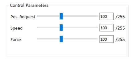
Fig. 5-3: Changing the Control Parameters of the Gripper
