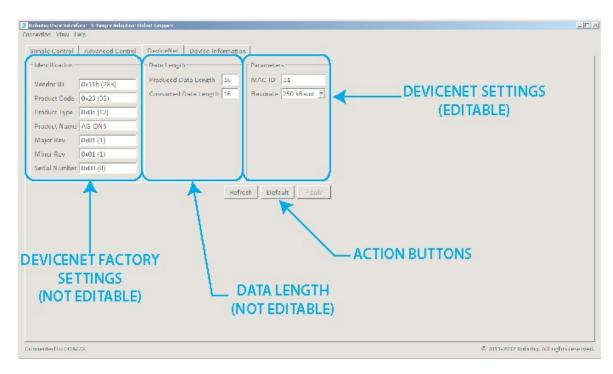
Fig. 6-6: Default screen of the Configuration Tool with DeviceNet
