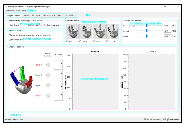
Fig. 5-1: Gripper Simple Control tab description.
