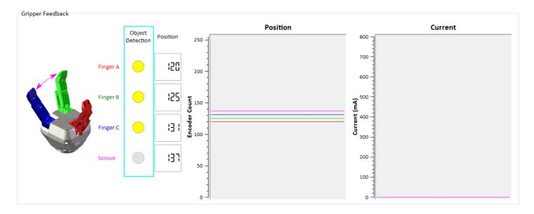
Fig. 5-4: Positive object detection is registered when the object detection dot turns yellow.
