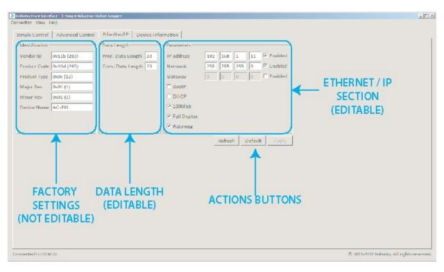
Fig. 6-3: Default screen of the Configuration Tool with Ethernet/IP
