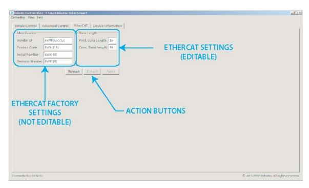
Fig. 6-5: Default screen of the Configuration Tool with EtherCAT
