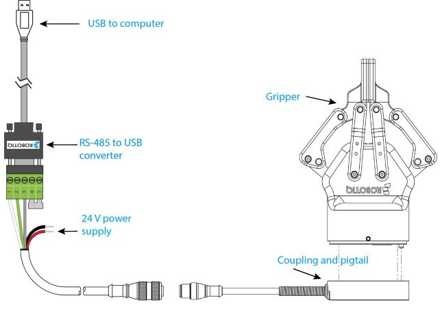
Fig. 3-6: Completed USB connection of the Gripper.
