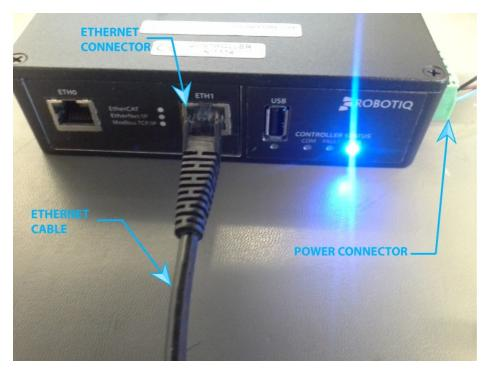
Fig. 3-8: Modbus TCP cabling setup for Adaptive Robot Gripper and Vacuum Gripper Series.
