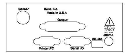
The SciCon back panel provides interfacing ports for:
