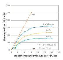
Fig. 1 - Transmembrane Pressure vs. Permeate Flux
