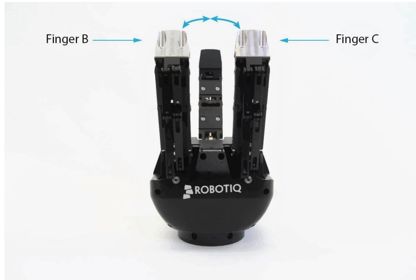
Figure 1.2 : First type of movement for the 3-Finger Adaptive Robot Gripper: changing the Operation Mode.
